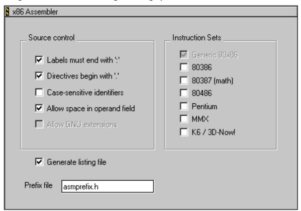
You can use the x86 assembler to generate code for several different instruction sets that are available for x86 processors. The Instructions Sets group of the Assembler target settings panel includes the following checkboxes, which you can select to indicate the instruction sets you want to use:
