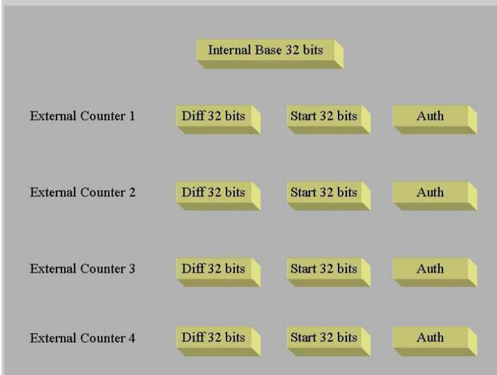
The internal base (IB) always moves forward and can never be reset. IB drives all external counters on the machine..
